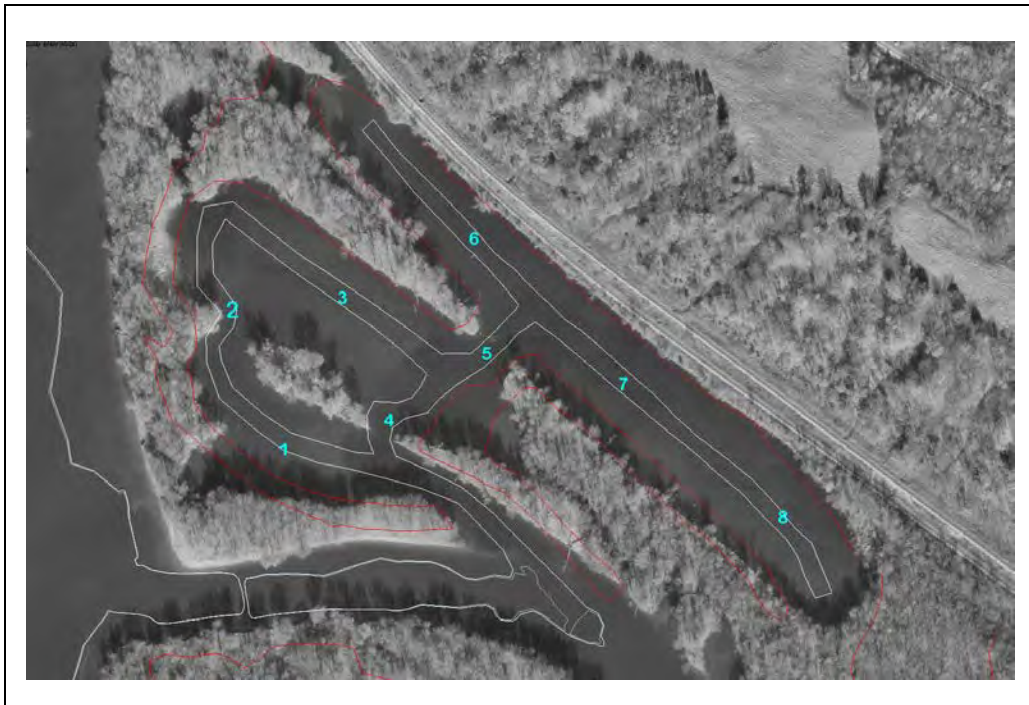
Figure H-2. Stone Lake Project Feature and Sub-Areas Used for Hydraulic Calculations
